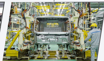
Body welding line
