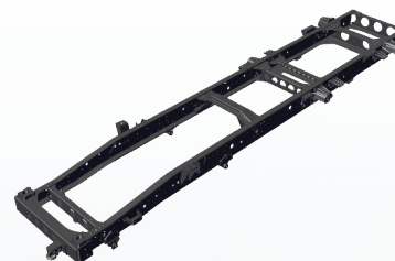
Chassis frame components
