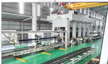
1,600-ton stamping line for exterior steel sheet components of chassis beams.
