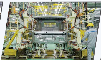
Body welding line
